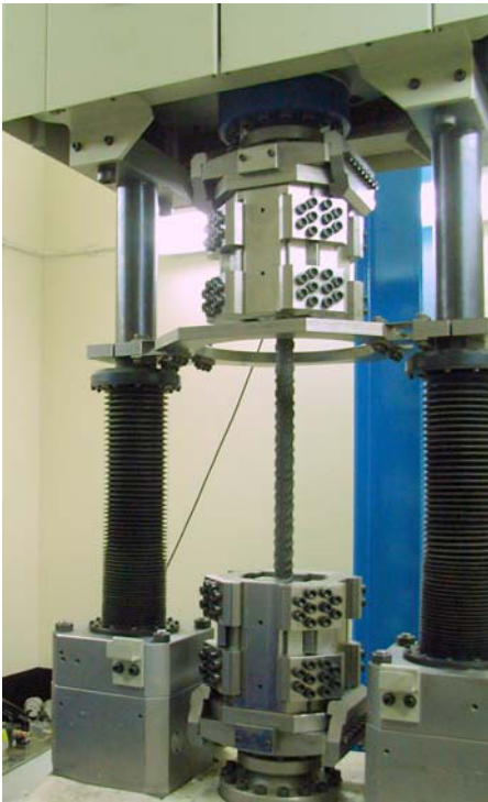
Tests on rebars with hydraulic clamping device PowerGrip 500 kN
