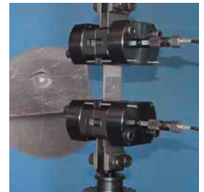
RUMUL HydroGrip with joining technology test sample
