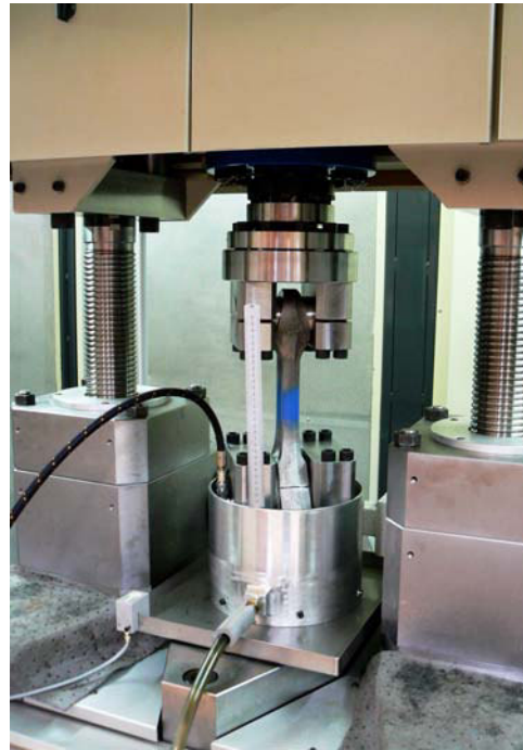
Tests on flat specimen with hydraulic clamping device HydroGrip 500 kN
