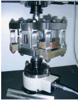
4-point-bending device resp. 8-point-bending device according to ISO 12108
